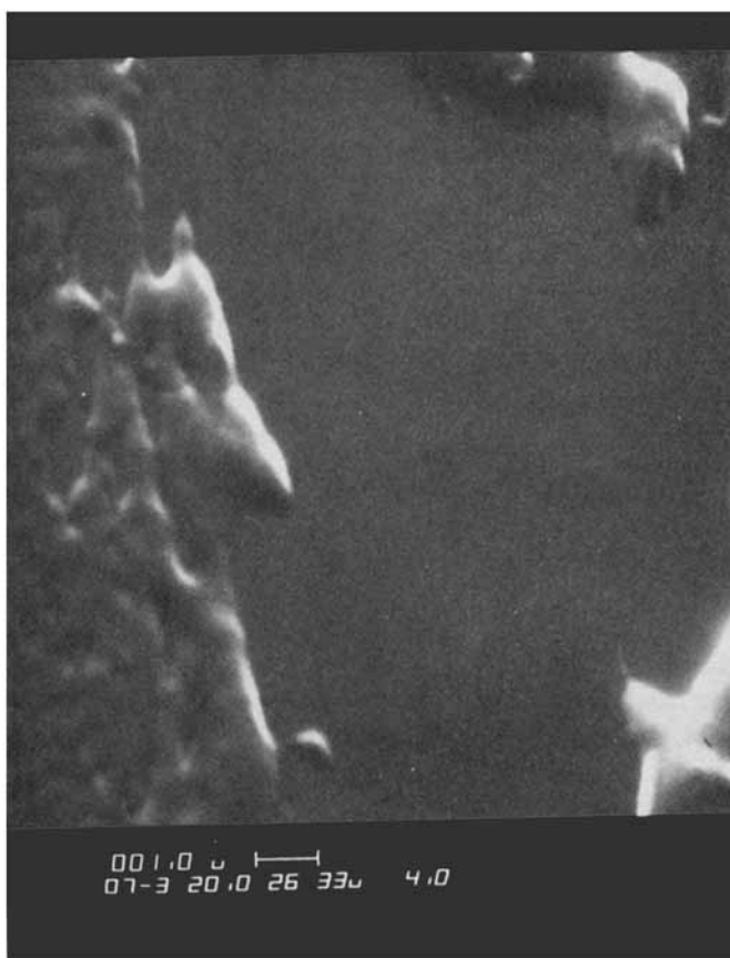
Fig. 7. SEM micrograph of scratches formed by a stainless steel probe (0.8 mm radius) on the spray-coated PDMS.
